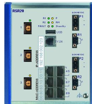
RSR20 09 00 JJ M3 T1 3x 100BASE-FX(MTRJ) 6x 10/100BASE-TX(RJ45)
