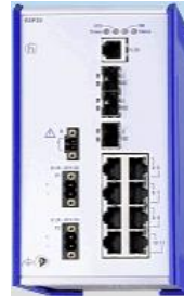
RSP3X 08 03 306 TT 3 SFP (GE/FE) 8x FE ports, RJ45
