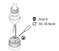
Unscrew the PE-contact, insert the PE-conductor and tighten again.
