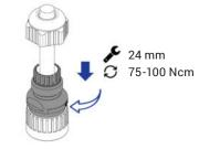
Screw the connector body to the contact holder.
